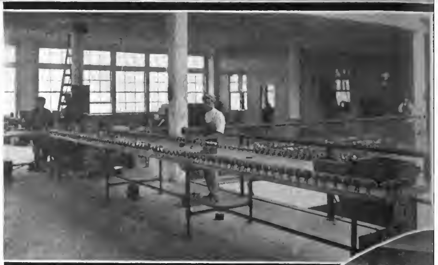
Showing Rows of Float Bowls on the Testing Benches Having the Buoyancy of the Floats Determined
